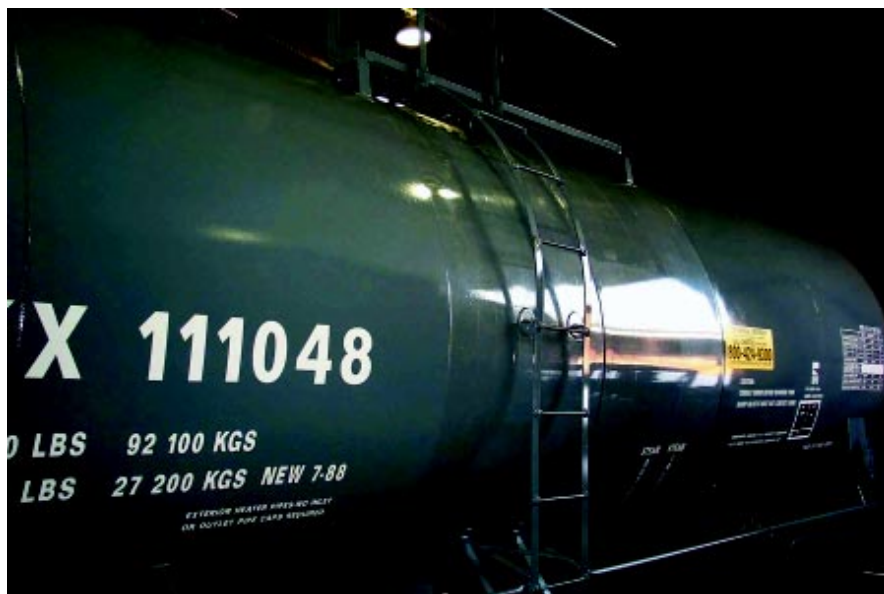
Rail car for sodium hydroxide (NaOH) has center-band coated with clear 5-mil ECTFE for paint protection, ease of cleaning, and minimized product buildup.
