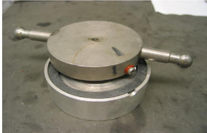
**Figure 3 – Desorption Test Cell**
