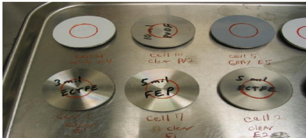
**Figure 6 – CARC Samples with  $5\text{cm}^2$  Wax Ring**
