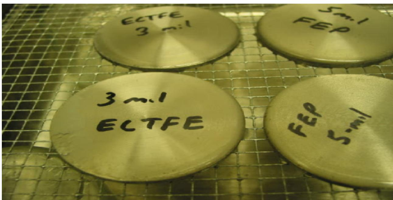
Photos 10 – Suspected peeling of film from E1 during DS2 residence (coating did not peel)
