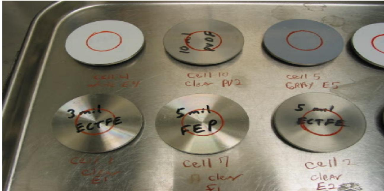
Photos 16 – Pretest photo: E1, F1, E2 (Front) – E4, PV2, E5 (Back)
