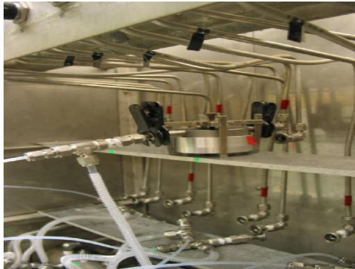
**Figure 4 – Cell Loaded into Desorption Test System**
