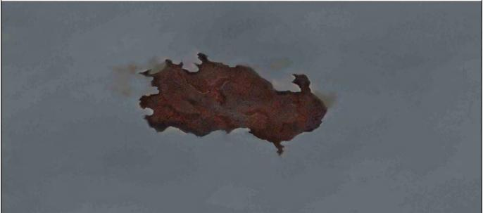
*FluoroGrip*® is used as a repair and maintenance system designed to extend the life of traditional coating systems by repairing damaged and rusted areas while they are small.
